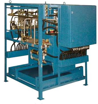
Frame-type power unit for 3 forging presses: 12 clamping circuits with pressure reduction for temperature compensation high pressure 4.2 l/min., 400 bar cooling return flow: 45 l/min., 10 bar
