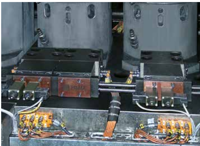
Wedge clamps with directly manifold-mounted directional control valves
