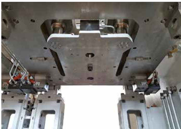
Wedge clamp on the press ram
