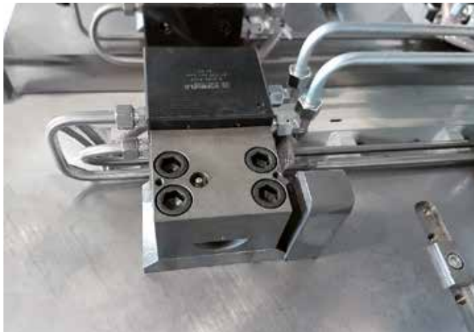
Wedge clamp with hydraulic ports A+B at the right and an additional cooling circuit C+D at the opposite, left side
