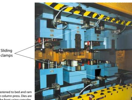
Sliding clamps fastened to bed and ram of a double column press. Dies are entered from the front using consoles.
