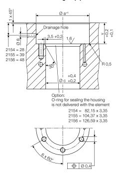
Manifold-mounting connection requires a plain and neat surface. The drainage hole may be drilled in any position provided that spray and separating agent can drain off freely.
