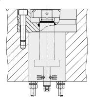
Pipes are recommended in applications where fittings are easily accessible and where pipes do not impede installation and dismantling of the swing sink clamps.
