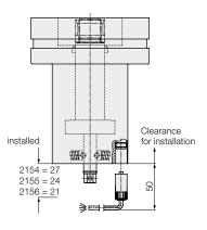
The three proximity switches are connected to the base of the swing sink clamp through a connecting cable with a screw coupling [IP 67]. (The connecting cable is not included in the delivery).
