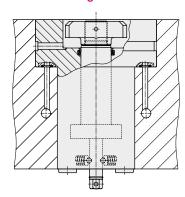
Hydraulic oil is fed through the drilled holes in the bed and in the ram. There are no exposed pipes or fittings. The sealing is made by O-rings supplied with the clamping element. Easy installation, ease of servicing
