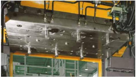
Use of swing clamps in the press ram. Shown is the die change position, i.e. the ram is in the upper position and the swing clamps are extended.
