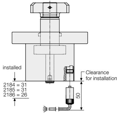
Both proximity switches are connected to the base of the pull clamp through a connecting cable with screw coupling [IP 67]. Please order the connecting cable separately. Further installation may be carried out using a distribution board with an LED display.
