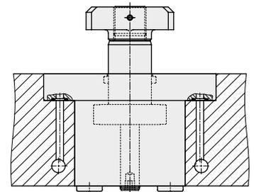
Hydraulic oil is fed through the drilled holes in the bed and in the ram. There are no exposed pipes or fittings. The sealing is made by O-rings supplied with the clamp. Easy installation, ease of servicing.
