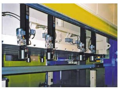
Rapid clamping system with pusher chain fastened to the press ram of a double column press. A hollow piston cylinder serves as clamping element.
