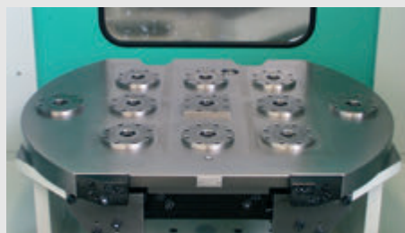
Square SPEEDY classic 1 STANDARD for single mounting (positioned secured against turning)
