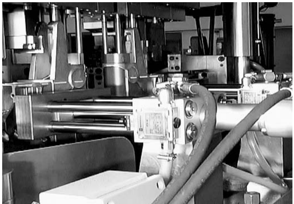
Application of the RS hydraulic slide on a deburring tool
