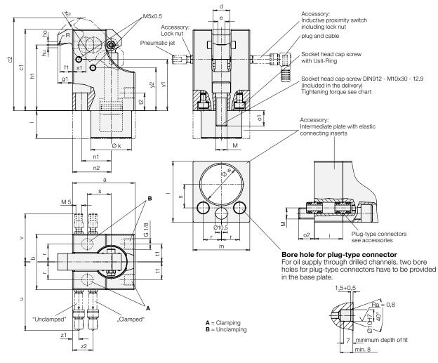
For manifold mounting, remove socket head cap screws with USIT rings and 2 screw-in plugs G 1/8 in the body.
