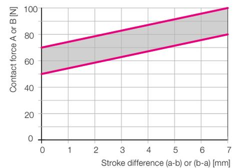
Diagram valid for horizontal mounting position. For vertical arrangement the weight of the clamping jaws has to be considered.
