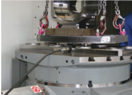
DMU 100: optical release check – „Thank heavens for hydraulics!“ The Speedys lift the pallet on release. Thus safe handling is guaranteed.
