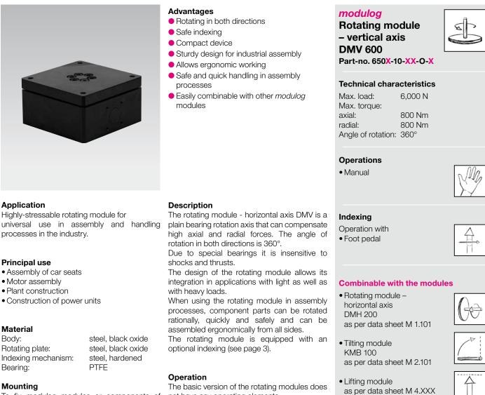
To fix modulog modules or components of the user, the rotating module has a 140 x 140 modulog interface in the flange plate and the body.
